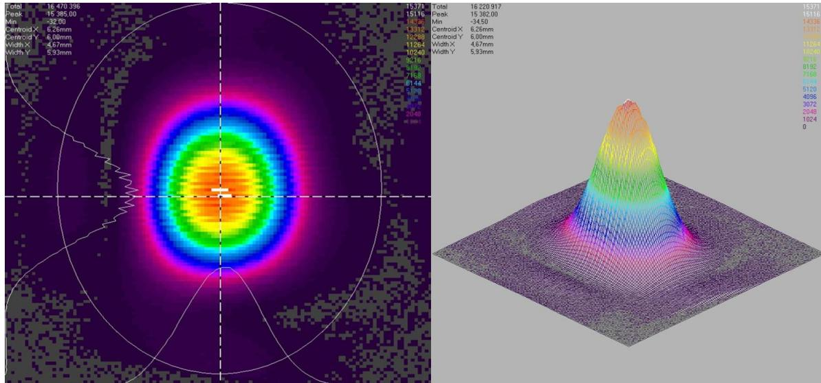
Figure 6. 2-D and 3-D beam profiles at 11P(20) line.
