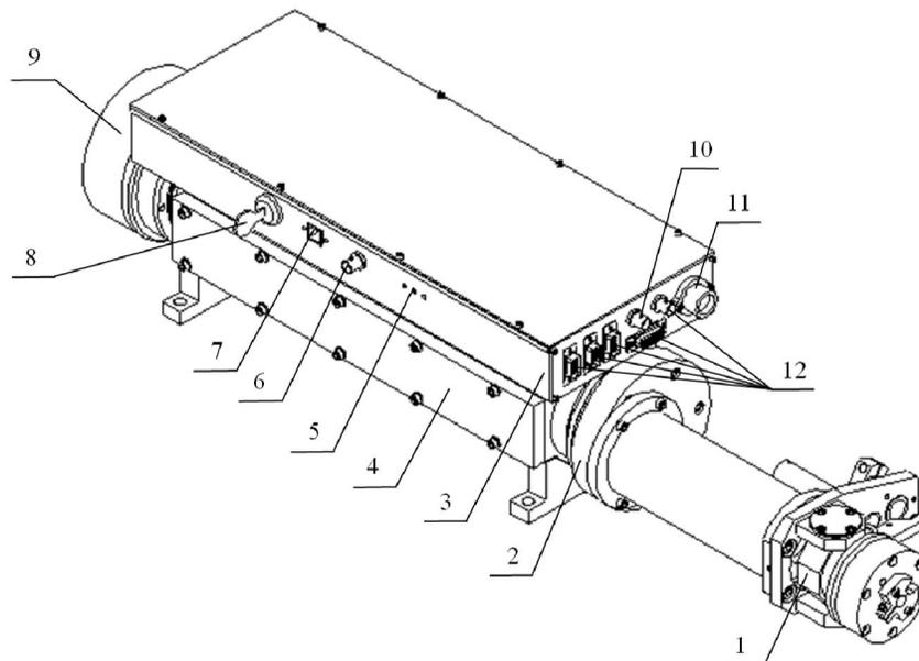
Figure 1 — Outer view, where: 1 — lasing line tuning unit; 2 — laser head body; 3 — electronic control unit combined with RF exciter (ECU); 4 — air/liquid heat exchanger; 5 — operation mode LED indication; 6 — synchronization signal OUT socket; 7 — USB B socket for PC control; 8 — safety key; 9 — power meter unit; 10 — power meter signal OUT socket; 11 — power cable socket; 12 — service sockets.
