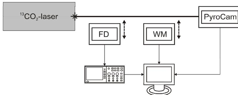
Figure 4. Scheme for measuring the main parameters of the tunable CO<sub>2</sub>-laser in working wavelength range, where: FD – fast detector (Vigo system PVM-10.6); WM – Wave length Meter (Angstrom WS6-200 IR-III); PyroCam - laser beam analyzer (Ophir Spiricon Pyrocam III)
