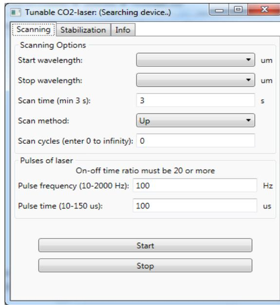
Figure 3. "Tunable CO<sub>2</sub>-laser" software main window screenshot.
